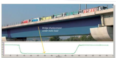
Dynamic monitoring : real-time displacement of two reflectors
