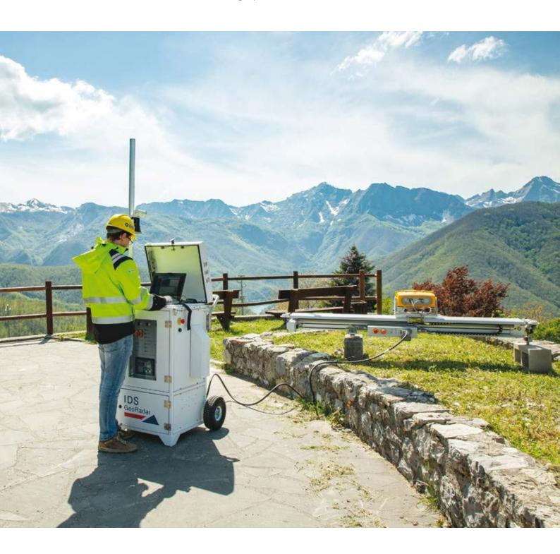
Next generation long-range radarfor slope and structural monitoring
