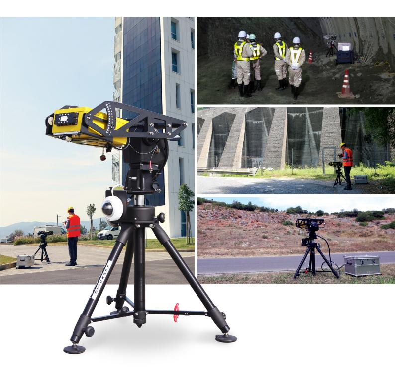
High-resolution radar system for early warning and real-time monitoring of buildings, dams, tunnels, mining infrastructures, and cut-slopes.
